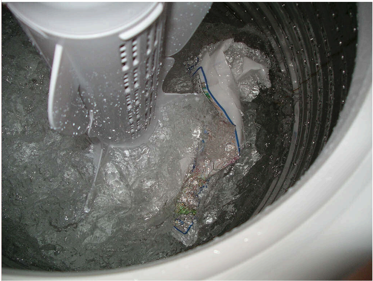
Illustration 1: GW512 Orienteering wet weather simulator for testing maps on synthetic substrates
